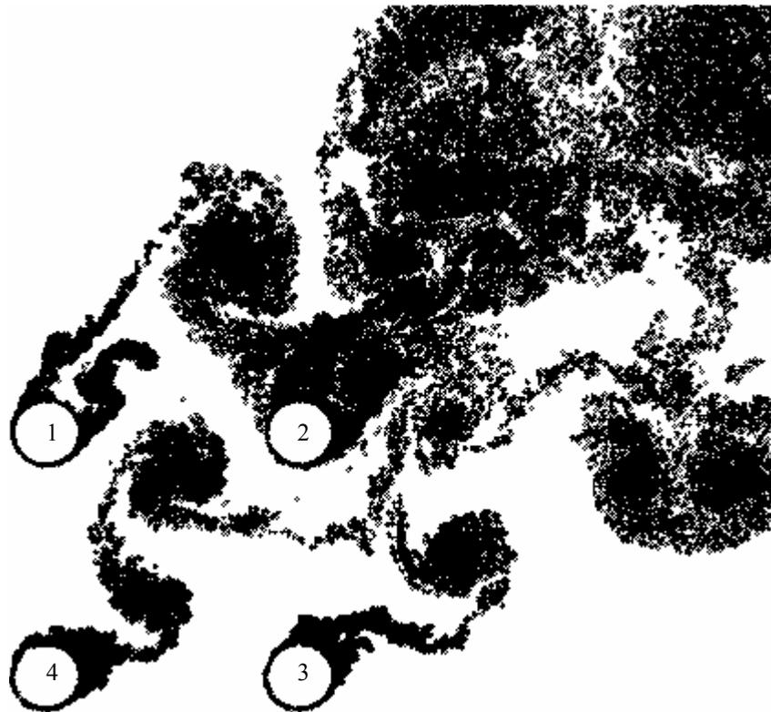
Figure 5. Position of the wakes vortices at  $t=60$  for  $L/D=4$ ,  $\alpha=45^\circ$ ,  $Re=1.3 \times 10^4$ ,  $\varepsilon=\sigma_0=0.03b$ ,  $\Delta t=0.05$ ,  $M=50$ .
